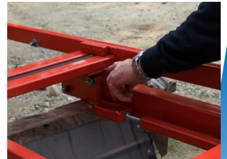
4. The angle can be set by placing a thickness gage block of desired thickness on the positive stops by the bell cranks
