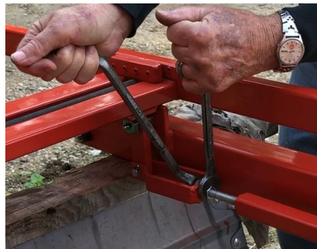
7. Move adjustable bell crank against the tilt table
