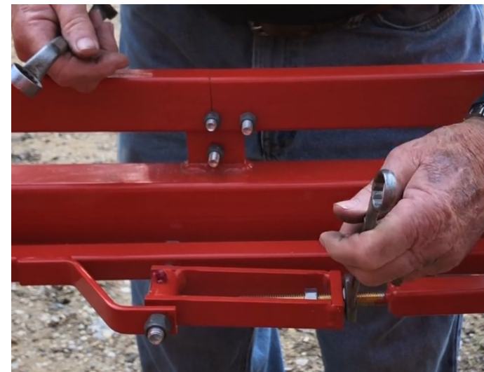
3. Snug nut against push rod clevis until the desired angle is attained
