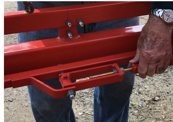
3. Loosen jam nuts at the push rod clevis
