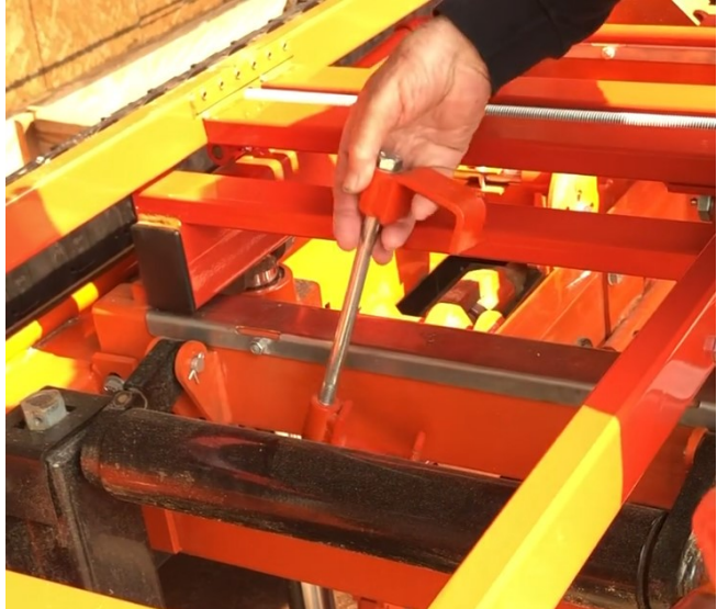
4. Using the Bevelsider mounting clamps, place the top of the clamp over the Bevelsider base crossmember and the bottom clamp over the sawmill support beam
