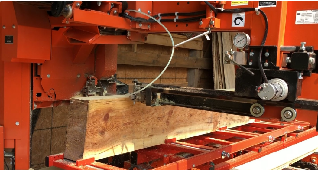
2. Using the patented clamping system and an electric driver with a 15/16" socket, clamp your siding cant in the Bevelsider
