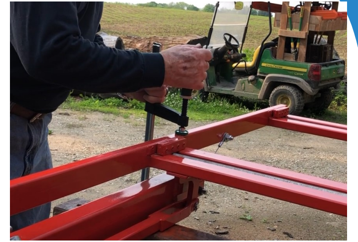
2. Clamp tilt table to base frame
