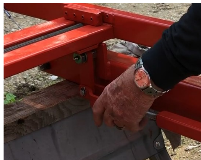
8. Snug nut up on adjustable bell crank clevis
