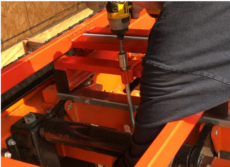
4. Using the Bevelsider mounting clamps, place the top of the clamp over the Bevelsider base crossmember and the bottom clamp over the sawmill support beam
