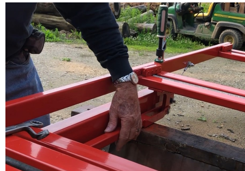
4. Move push rod so non-adjusting bell crank is against the bottom of the tilt table
