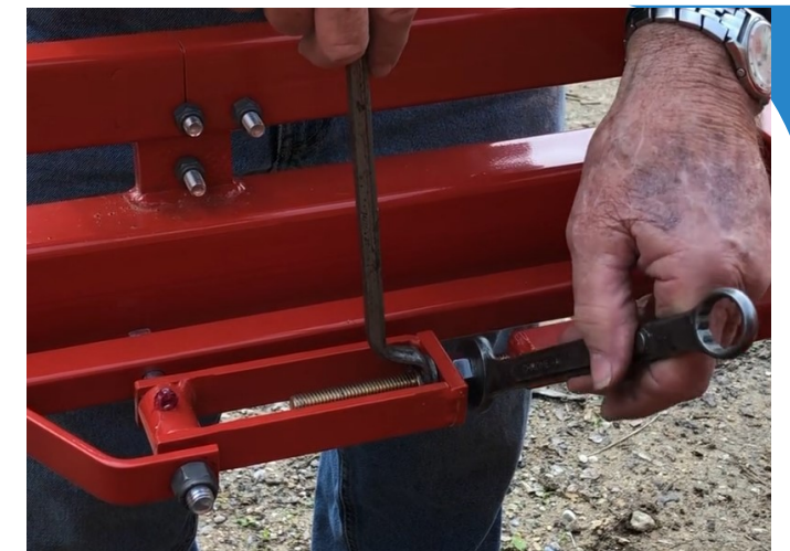
2. Once bell cranks are timed, using two 3/4" wrenches, loosen nuts at push rod clevis
