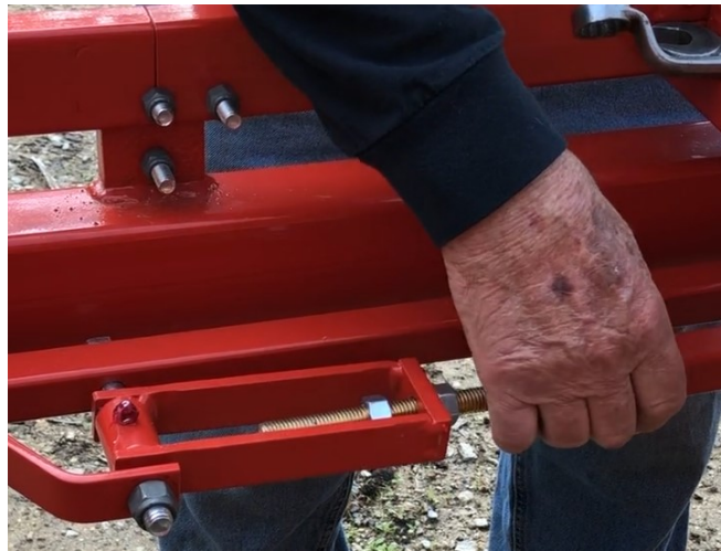
5. Run nut of push rod against push rod clevis
