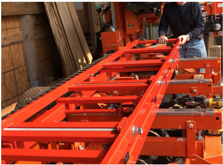
3. Line Bevelsider base crossmembers with sawmill support beams
