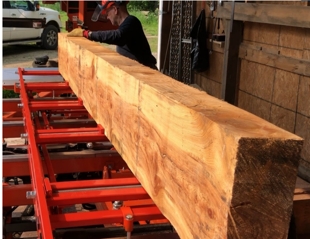
2. Using the patented clamping system and an electric driver with a 15/16" socket, clamp your siding cant in the Bevelsider
