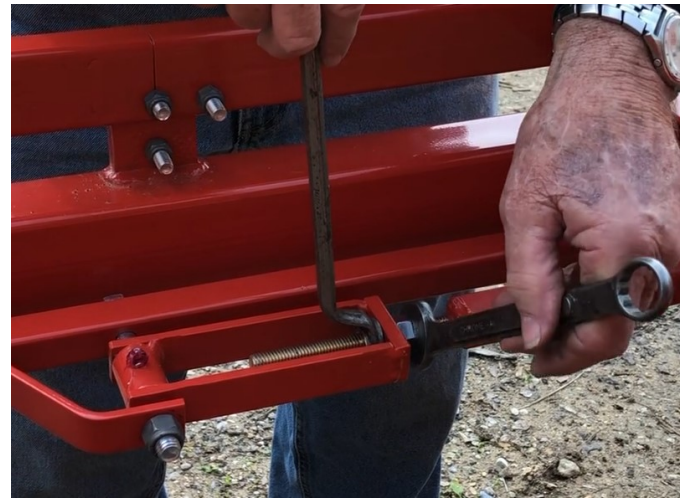
6. Using two 3/4" wrenches, tighten jam nut on push rod clevis
