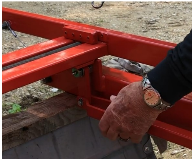
7. Move adjustable bell crank against the tilt table
