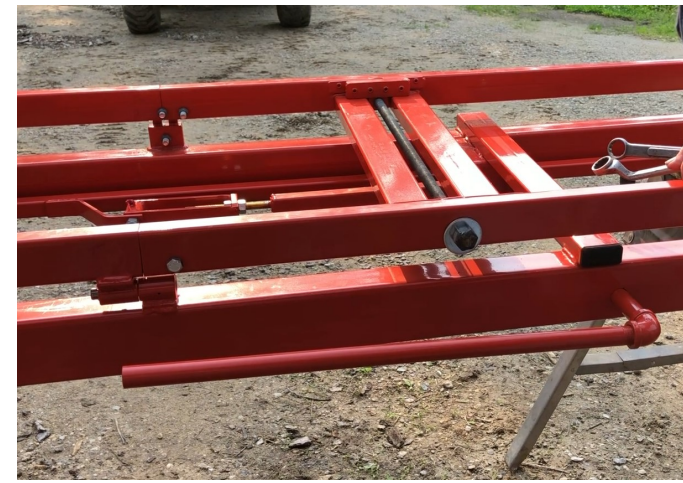
1. Tilt table handle must be in the up position
