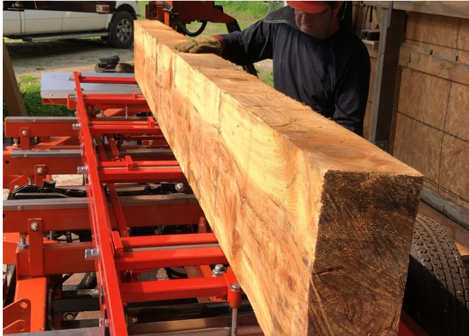
1. Place you siding cant on the Bevelsider
