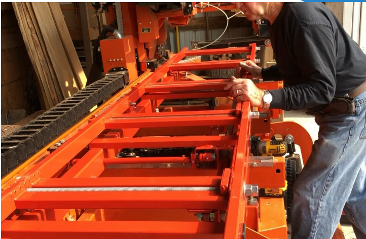
2. Push the Bevelsider up against the sawmill side stops
