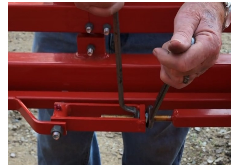
5. Adjust height until gage block slides between bottom of tilt table and positive stop
